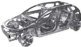
These steels are characterized by low carbon and alloy element contents, which gives them excellent functional properties such as suitability for welding or coating. Their hardening obtained by precipitation and grain size refinement makes it possible to achieve high levels of mechanical resistance. They combine improved weldability and good formability.
